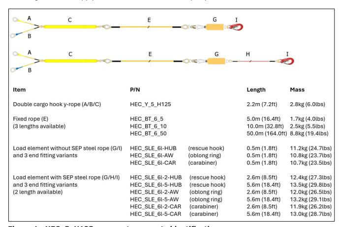
Figure 1: HEC\_5\_H125 rope system - parts identification
