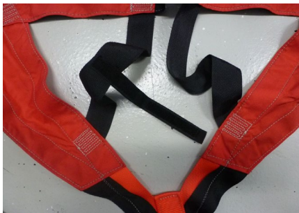
Fig. 9: Reinforcement strap sewn onto left bottom belt
