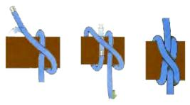
Schematic illustration of a clove hitch:
