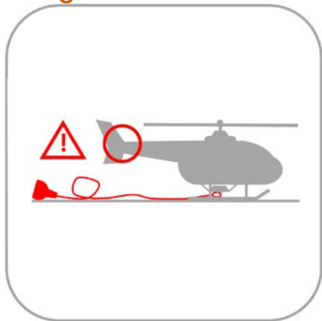
HAZARD: TAIL ROTOR NEAR ROPE LOOPS
