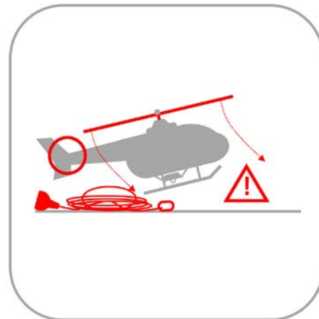
HAZARD: LANDING FLARE ABOVE ROPES
