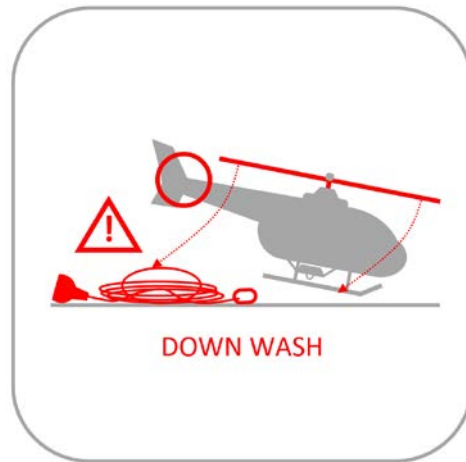
HAZARD: DOWN WASH AND TAIL ROTOR
